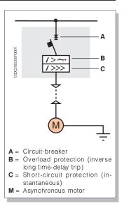
Diagram showing direct starting of asynchronous motor using only the circuit-breaker fitted with a microprocessor-based overcurrent release.
