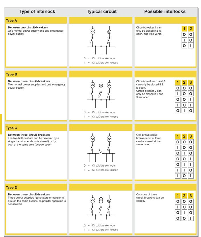
The emergency power supply is usually installed to take over from the normal power supply in two instances:
