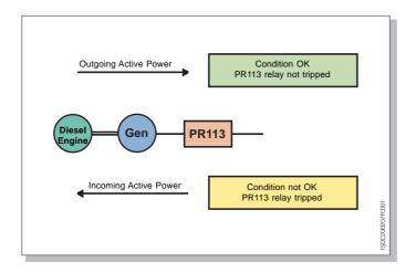
When the power measured by the relay falls below zero, the PR113 release trips, opening the circuit-breaker and thus preventing damage.
