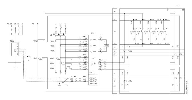
Three-pole circuit-breaker with PR111, PR112/P, PR112/PD, PR113P, PR113/PD microprocessor-based release and current transformer on neutral conductor outside circuit-breaker
