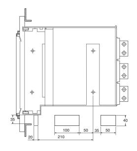
Tightening torque for fastening screws Nm 20 Tightening torque for main terminals Nm 70 Tightening torque for earthing screw Nm 70
