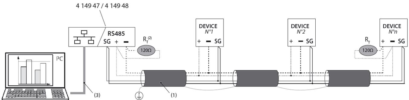
(1) RS485: Prescribed use of Cable Belden 9842, Belden 3106A (or equivalent) for a maximum length of 1000 m, or Category 6 cable (FTP or UTP) for a maximum length of 50 m;
