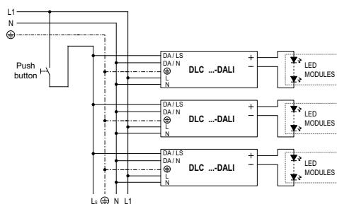
**Corridor function:** Dimming system that controls light level when a presence is detected by a conventional mains on/off sensor connected in DALI input. When the sensor detects a presence, light level increases up to 100%, otherwise the control gear keeps on providing 10% light level.
